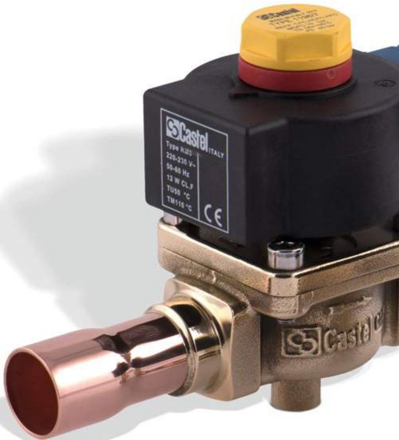
can be mounted in any position so long as the coil does not point downwards. The brazing of valves with solder connections should be carried out with care, using a low melting point filler material. It is not necessary to disassemble the valves before brazing, but it is important to avoid direct contact between the torch flame and the valve body, which could be damaged and compromise the proper functioning of the valve.
