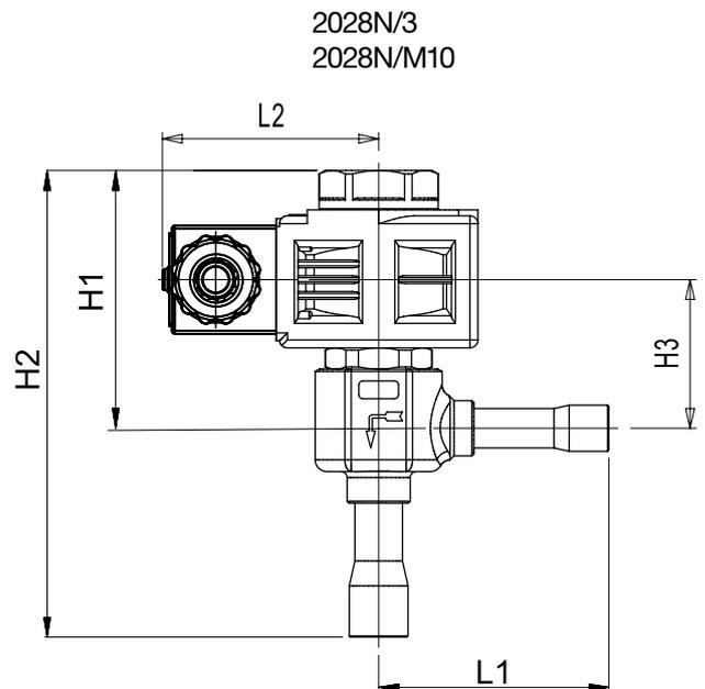
(1) : with coil 9300 the dimension L2 is equal to 34 and the weight must be decreased of 45 g
