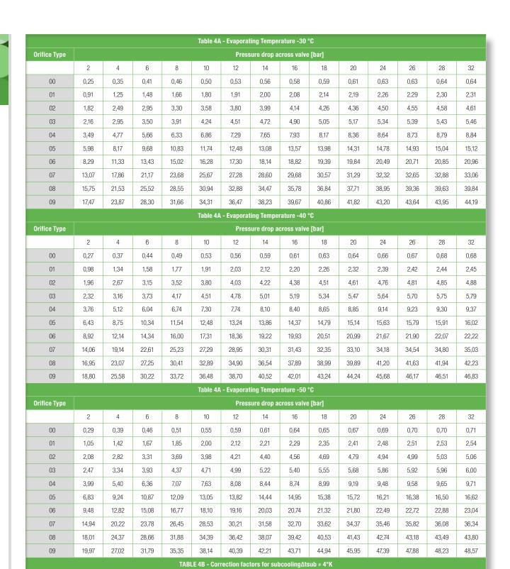
When subcooling ahead of the expansion valve is other than 4 °K, adjust the evaporatore capacity by dividing by the appropriate correction factor found in Table 4B
