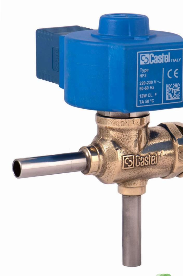
We recommend TIG welding for steel connectors of 1418E, 1428E and 1438E valves, to be performed as quickly as possible according to the method shown in the product instruction sheet. The connection material is AISI 304: it is only possible to use AISI 308 filler material if welding to pipes made from the same type of material. For pipes made from other materials, please contact your welding supplies supplier.
