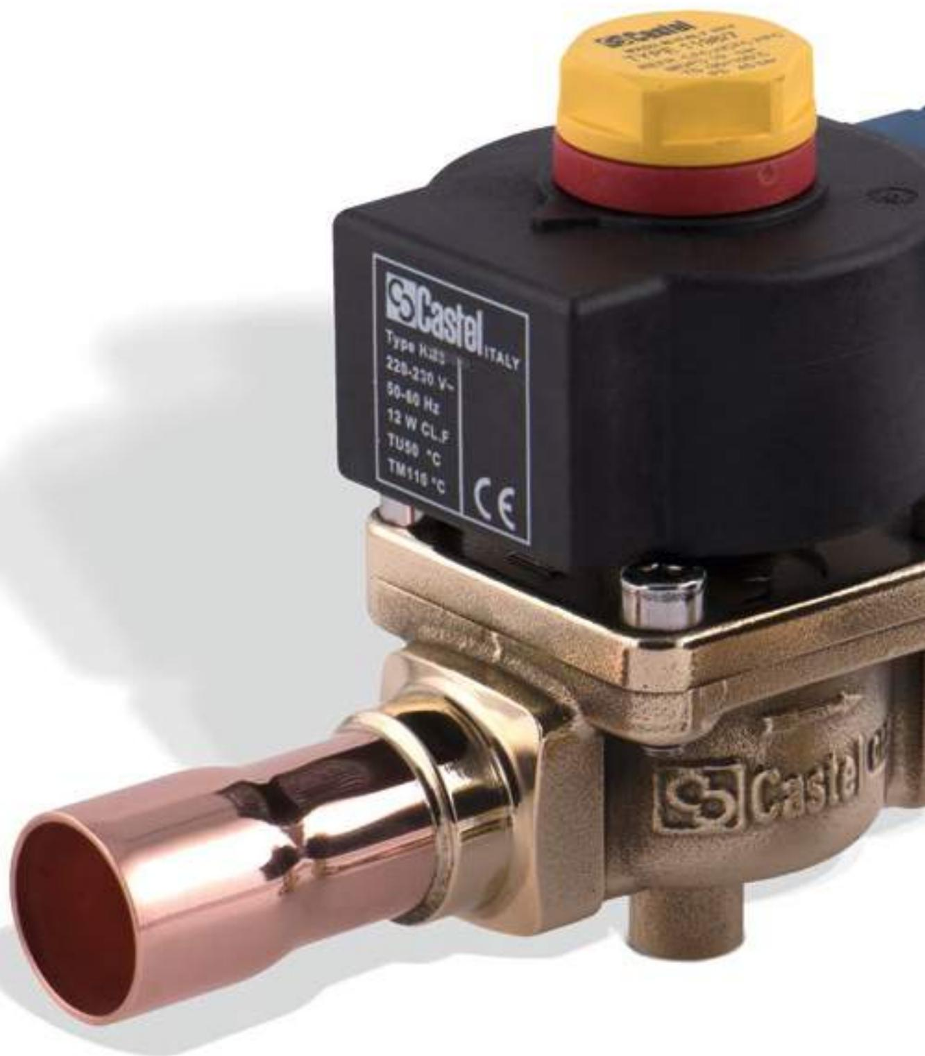
can be mounted in any position so long as the coil does not point downwards. The brazing of valves with solder connections should be carried out with care, using a low melting point filler material. It is not necessary to disassemble the valves before brazing, but it is important to avoid direct contact between the torch flame and the valve body, which could be damaged and compromise the proper functioning of the valve.
