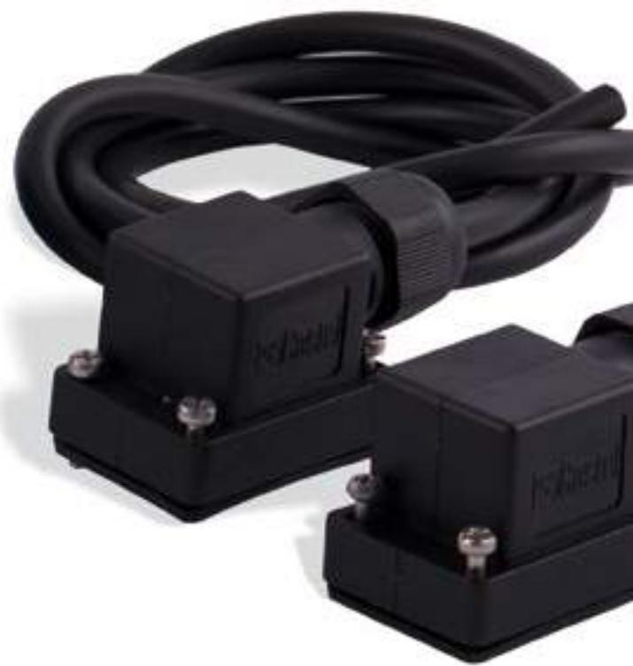
orientation of the outer casing with respect to the inner terminal block. The gland nut of the outer casing is suitable for receiving cables with an external diameter of 6 to 9 mm and is equipped with a self-locking device. Three-pole cables with a cross-section greater than or equal to 0.75 mm<sup>2</sup> are recommended.
